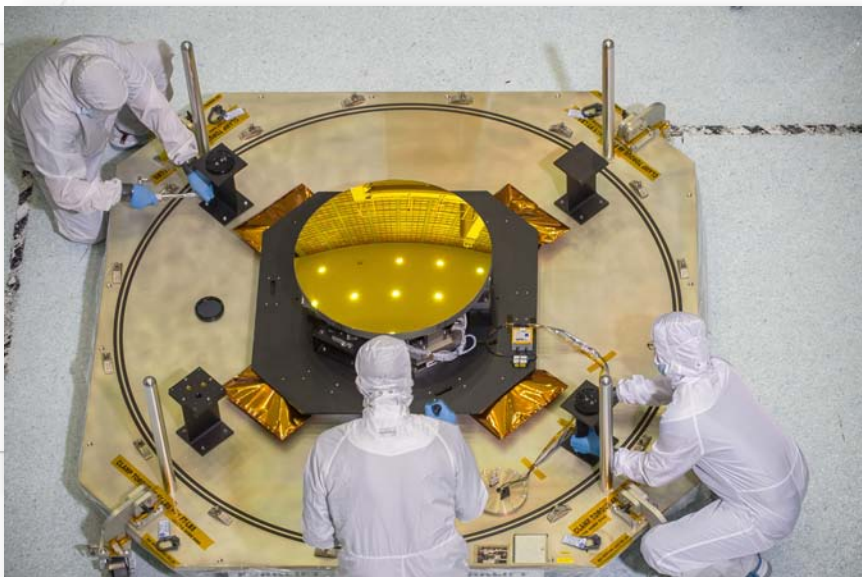
The flight secondary mirror undergoing receiving and inspection in the GSFC SSDIF Cleanroom.
