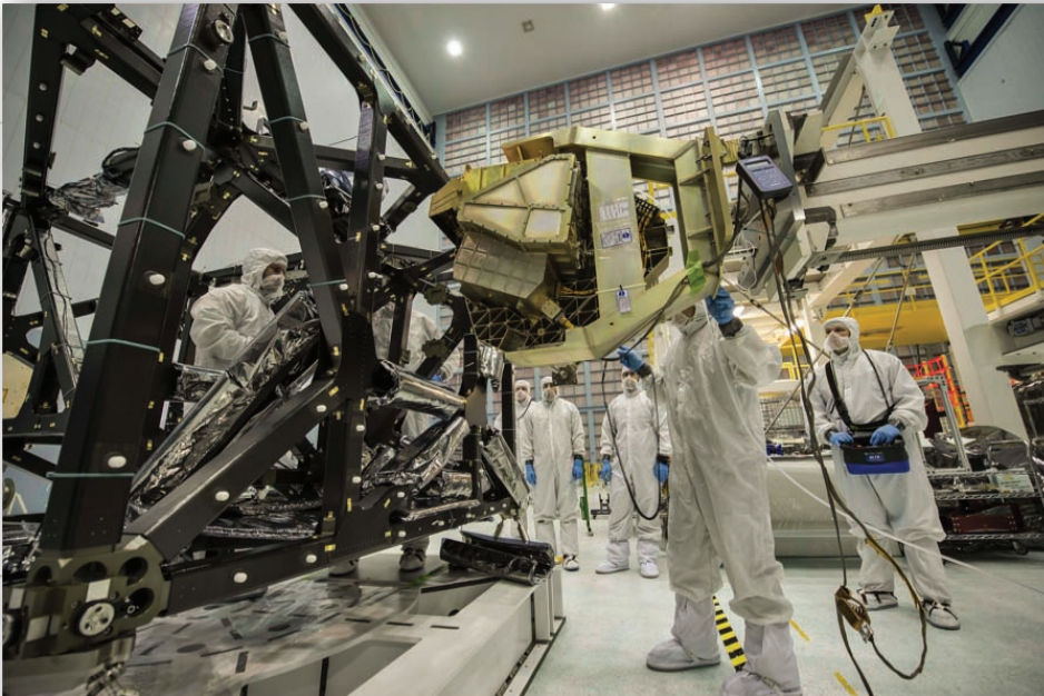
Figure 3: The flight FGS/NIRISS instrument is shown being integrated with the ISIM structure in preparation for the CV-1RR test.
