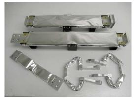
Figure 19: Proto-flight Heat Strap Segments
