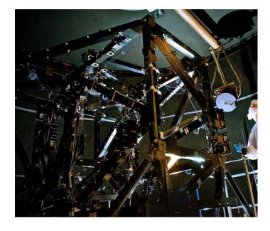
Figure 9: The ISIM flight structure in the SSDIF clean room (left); and in the space environment simulation chamber for cryogenic photogrammetric testing (right).
