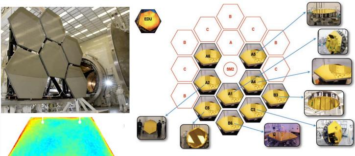
Above: JWST's optical train is rapidly being populated with completed mirrors. To date nine primary mirror segments have been gold-coated, including the flight spare EDU mirror. The flight tertiary and fine steering mirrors have also completed polishing and received their gold coating.
