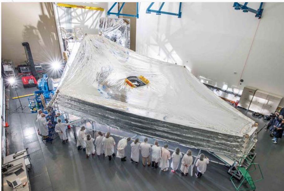
Figure 7. The 5-layer sunshield engineering model in its unfolded configuration after a deployment test at NGAS. Credit: NASA/Chris Gunn
